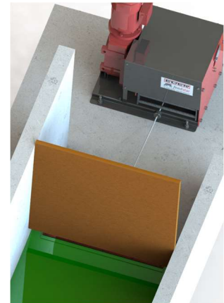
Fig. 27 Mounting wire and wire stopper
