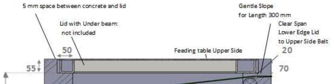
Fig. 8 Steel cover with under beam (optional)
