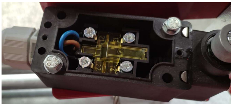
Fig. 37 Connection of limit switch
