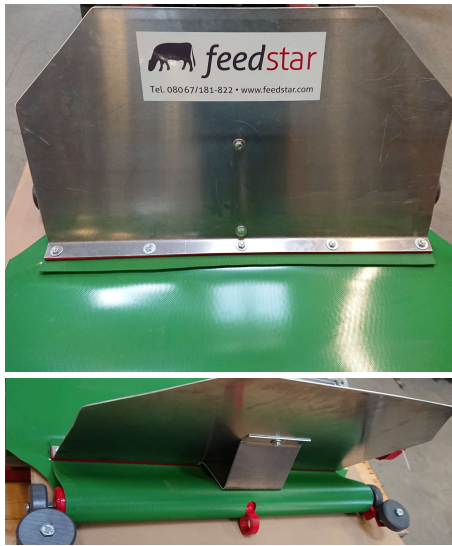
Fig. 31 Mounting shield pull bar
